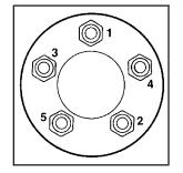
12. Tighten the wheel nuts firmly in a crisscross sequence, as shown.
